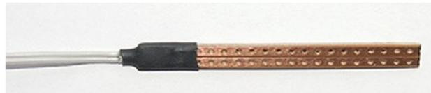
The copper lines are designed to be at the lowest part of the housing and facing the bottom of the housing, so that any moisture/water will immediately touch the copper lines. The opposite side of the copper lines has a sticker with our website name on it ([UWleakdetector.com](http://UWleakdetector.com)), this surface should be facing upwards in the housing.
