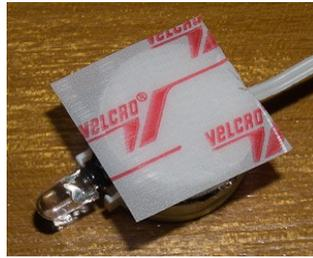
2. Remove just the adhesive backing tape from the second piece of 'velcro' on the Detector Circuit / LED assembly. But leave the second piece of 'velcro' in position on the back of the Battery Holder/Circuit/LED assembly).
